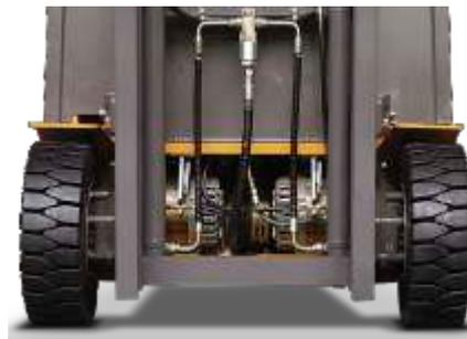
Twin AC motors are easily accessible from the front of the truck. Brushless AC means less servicing and fewer costly breakdowns.
