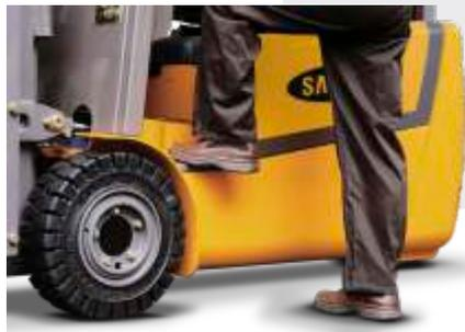
Wide steps allow the driver to mount the truck from either side - safely.
