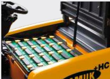
Accessible 48 volt batteries, standard and extra-duty, are controlled by CURTIS AC Gen2 circuitry and suit light or high-lift long shifts.
