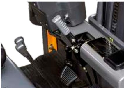
Toggle-action parking brake is dashboard mounted and can safely hold the truck on inclines of 16% or more.
