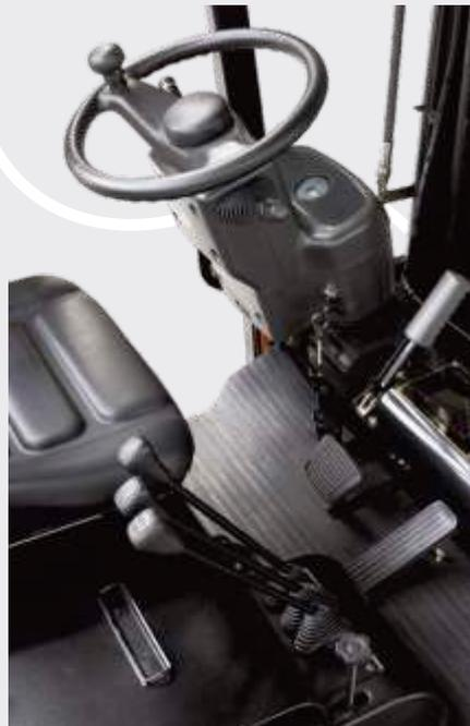
Simple instrumentation, a clear footwell and automotive-style controls help the driver feel at home, reducing stress and accidents.
